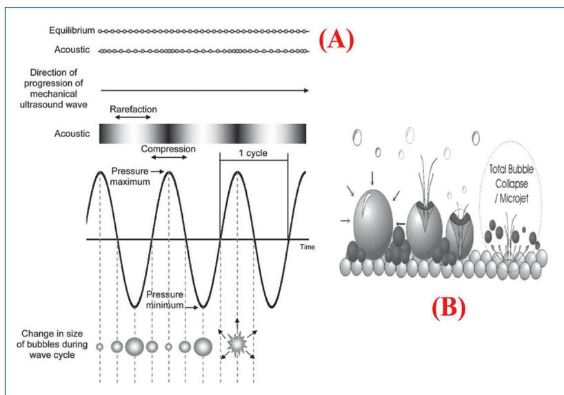
Figure 2: (A) Development and collapse of cavitation bubbles, and (B) schematic depicting classically thought bubble collapse at the solid surface <sup>112</sup>
