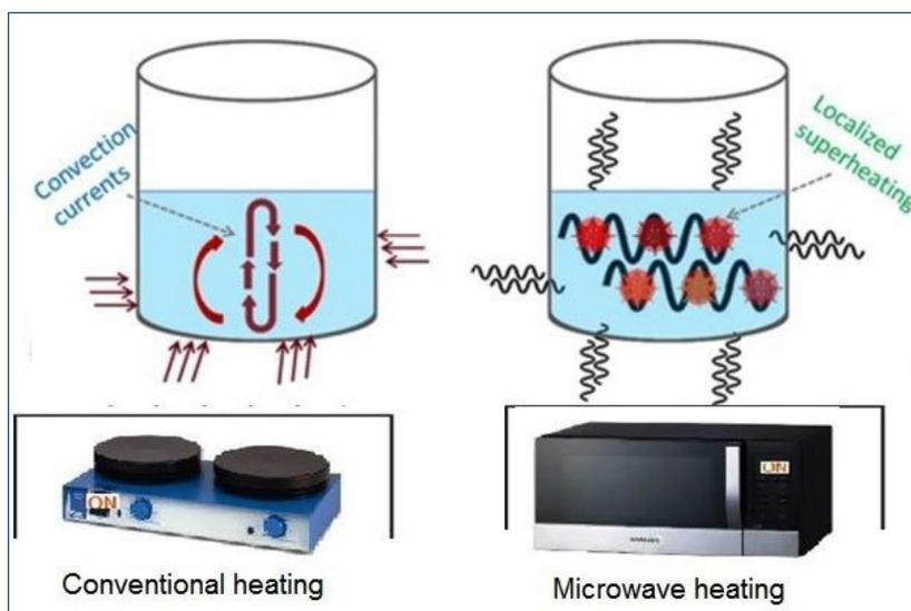
Figure 3: Conventional and microwave heating mechanisms
